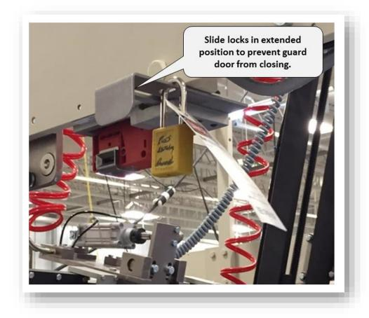
Being able to open the access panel and hang a lock on the slide gate enables the approved tasks to be performed without having to follow full LOTO procedures.
