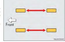
► Vehicles with front and rear tires of differing sizes Tires cannot be rotated.
