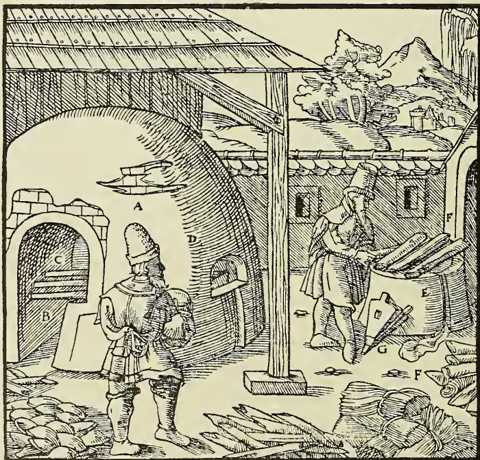
A—FURNACE SIMILAR TO AN OVEN. B—PASSAGE C—IRON BARS. D—HOLE THROUGH WHICH THE LITHARGE IS DRAWN OUT. E—CRUCIBLE WHICH LACKS A DOME. F—THICK STICKS. G—BELLOWES
