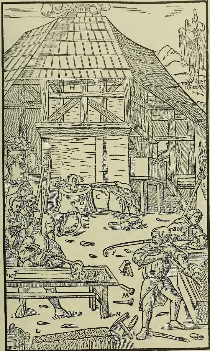
A—FURNACE. B—ITS TAP-HOLE. C—FOREHEARTH. D—ITS TAP-HOLE. E—SLUGS. F—SCRAPER. G—DIPPING-POT. H—WALLS OF THE CHIMNEY. I—BROOM. K—COPPER PLATE. L—LATTICEWORK BARS. M—IRON SEAL OR DIE. N—HAMMER.
