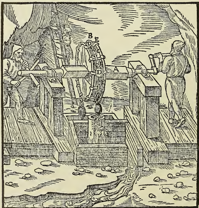
A—AXLE. B—DRUM. C—DRAWING-CHAIN. D—BALLS. E—CLAMPS.
