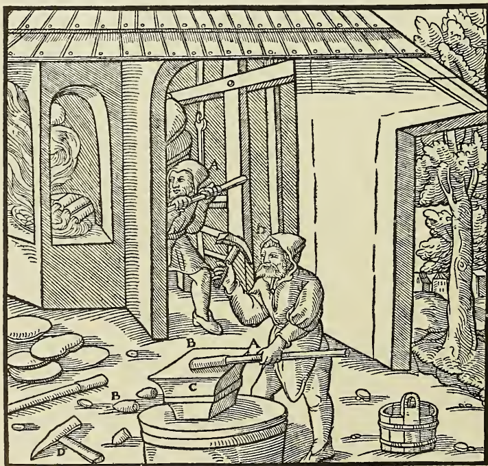
A—POINTED BAR. B—THIN COPPER LAYER. C—ANVIL. D—HAMMER.
