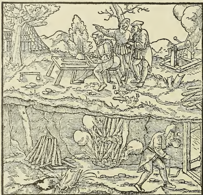
A—KINDLED LOGS. B—STICKS SHAVED DOWN FAN-SHAPED. C—TUNNEL.
