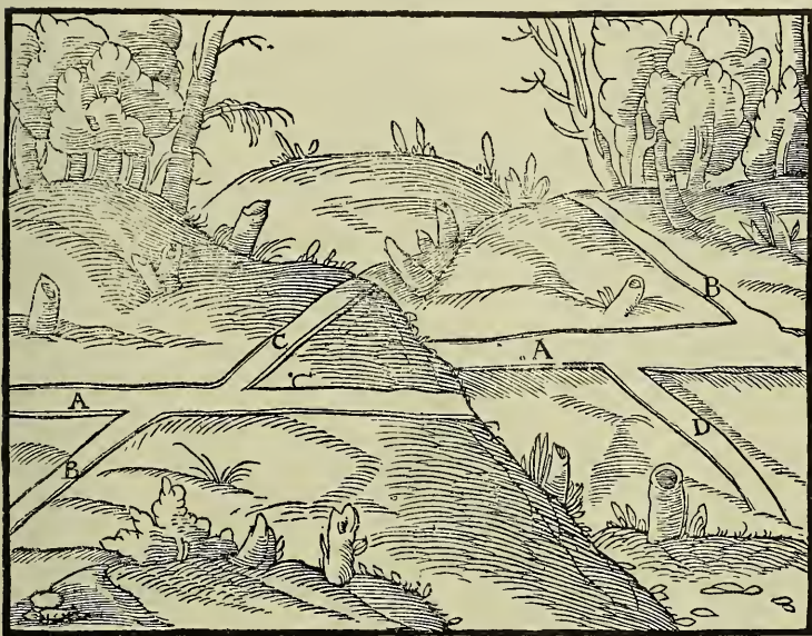
A—PRINCIPAL VEIN. B—VEIN WHICH CUTS A OBLIQUELY. C—PART CARRIED AWAY. D—THAT PART WHICH HAS BEEN CARRIED FORWARD.
