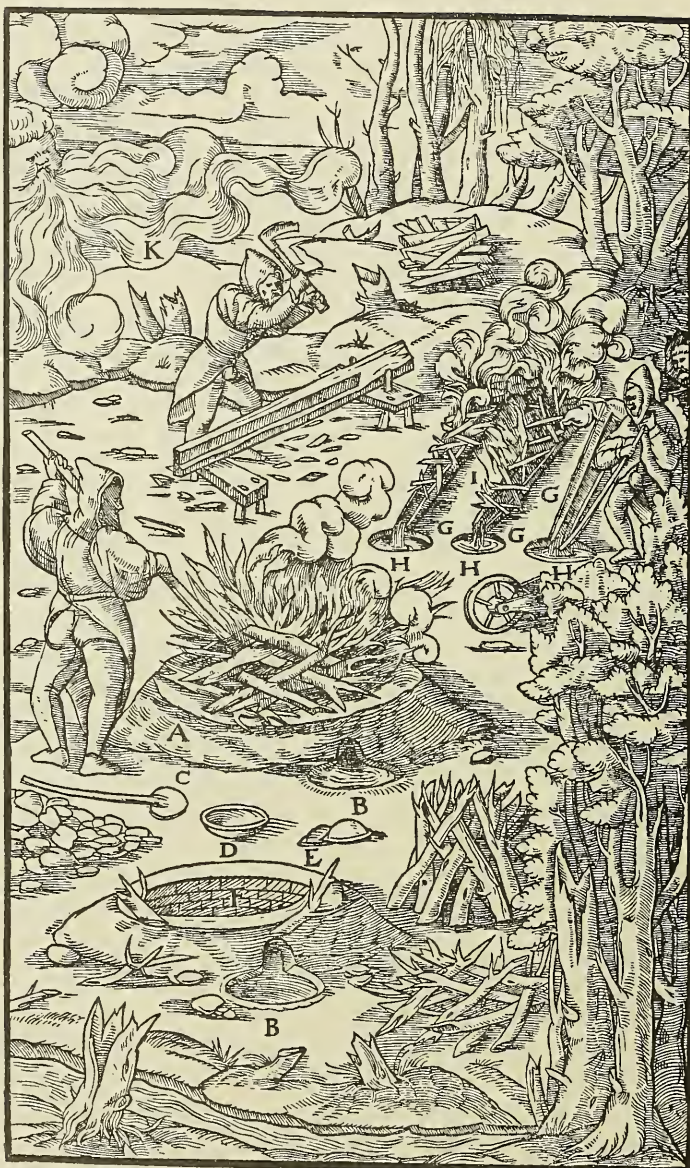
A—PIT ACROSS WHICH WOOD IS PLACED. B—FOREHEARTH. C—LADLE. D—IRON MOULD. E—CAKES. F—EMPTY POT LINED WITH STONES IN LAYERS. G—TROUGHS. H—PITS DUG AT THE FOOT OF THE TROUGHS. I—SMALL WOOD LAID OVER THE TROUGHS. K—WIND.
