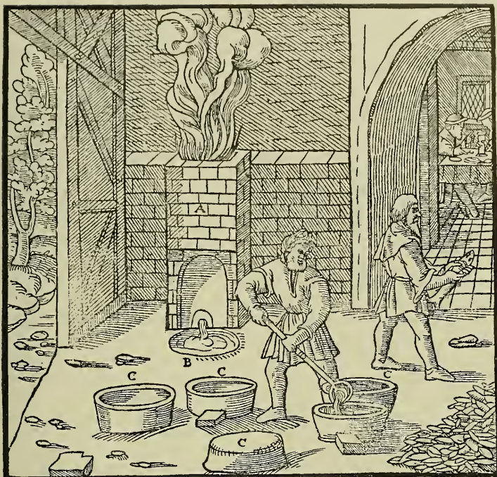
A—FURNACE. B—FOREHEARTH. C—OBLONG MOULDS.
