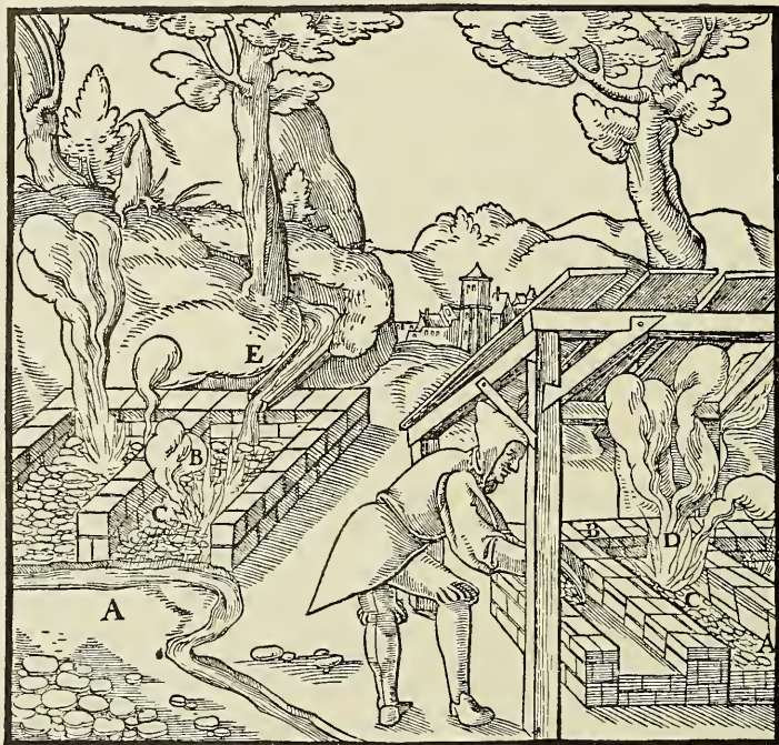
A—AREA. B—WOOD. C—ORE. D—CONE-SHAPED PILES. E—CANAL.
