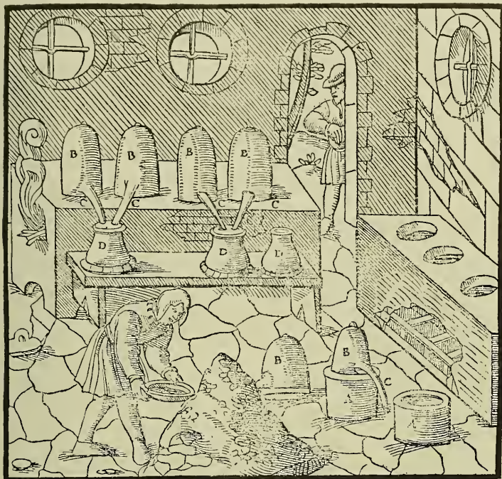
A—POTS. B—OPERCULA. C—NOZZLES. D—GOURD-SHAPED EARTHENWARE VESSELS.
