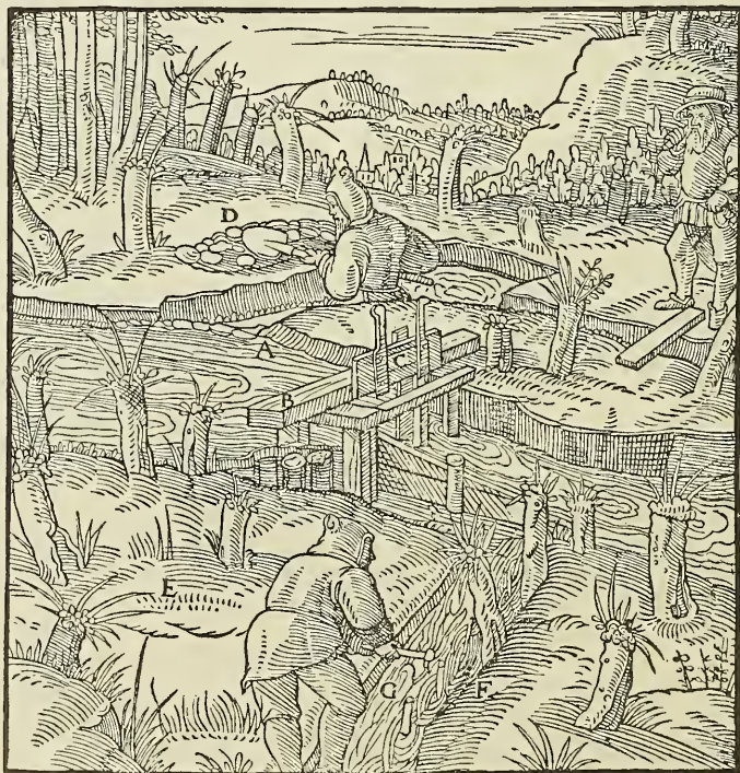
A—RIVER. B—WEIR. C—GATE. D—AREA. E—MEADOW. F—FENCE. G—DITCH.
