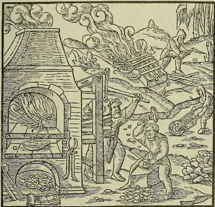
A—WOOD. B—BRICKS. C—PANS. D—FURNACE. E—CRUCIBLE. F—PIPE. G—DIPPING-POT.
