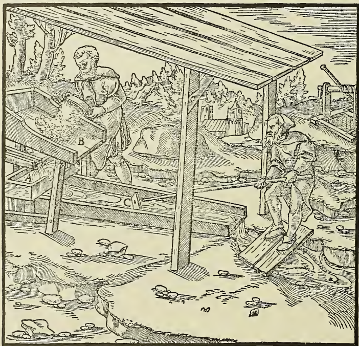
A—TROUGH. B—PLATFORM. C—WOODEN SCRUBBER.
