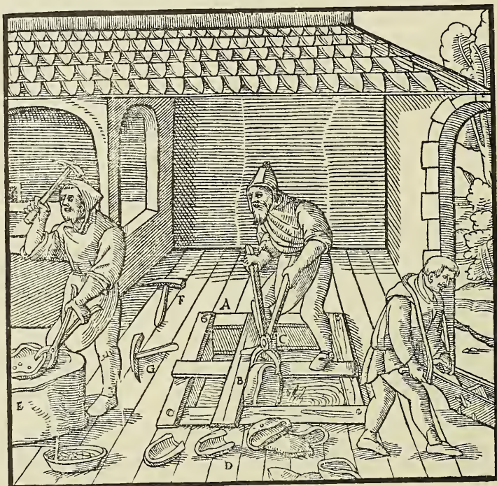
A—TANK. B—BOARD. C—TONGS. D—"DRIED" CAKES TAKEN OUT OF THE TANKS. E—BLOCK. F—ROUNDED HAMMER. G—POINTED HAMMER.
