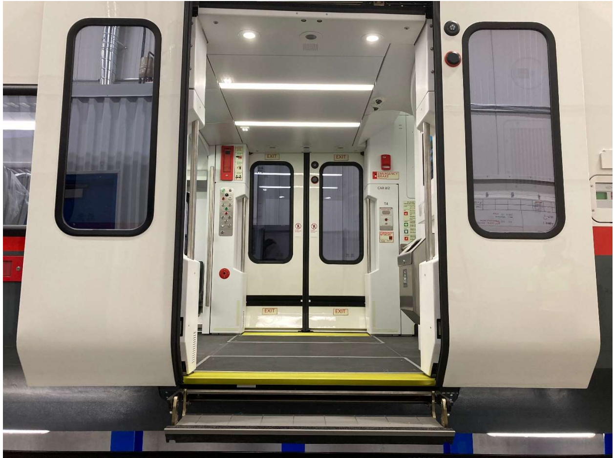
Figure F2 –Side Door Open with Step Deployed and Handholds Accessible
