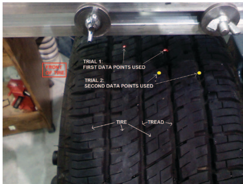
Figure 4-7. Locations of tread depth measurements of the tire cross section.
