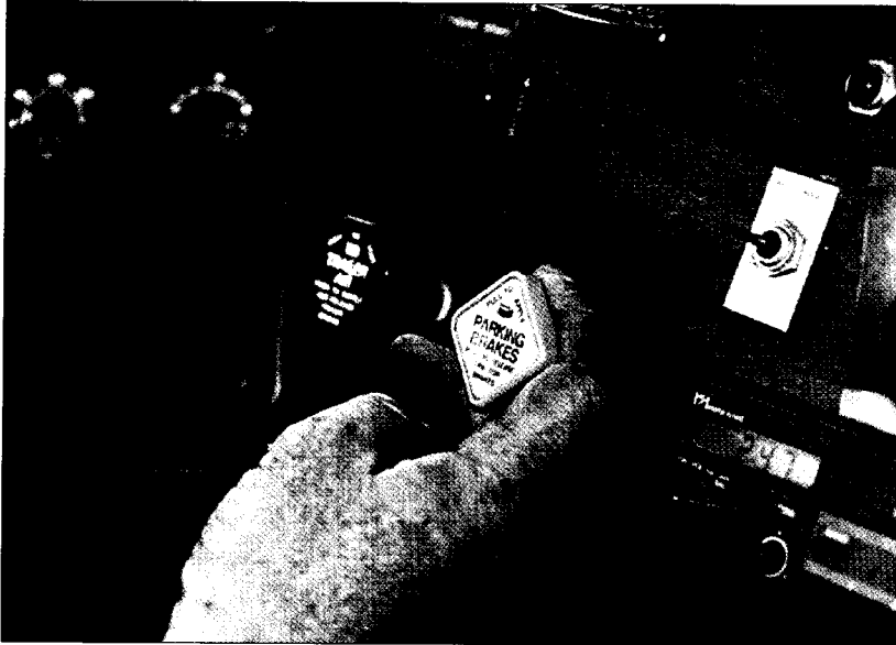
As illustrated, a typical two-valve tractor protection system restricts air flow to a trailer. In contrast, custom-spec'ing a three-valve system provides an extra dash knob, for sending air directly to the trailer after hook-up.
