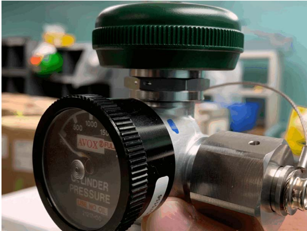
FIGURE 7 MARK ACCEPTABLE CVA WITH A BLUE PAINT DOT
