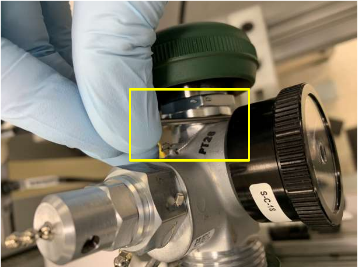
FIGURE 4 CLOSE-UP OF INSPECTION PROCEDURE LOCATION ON VALVE ASSEMBLY
