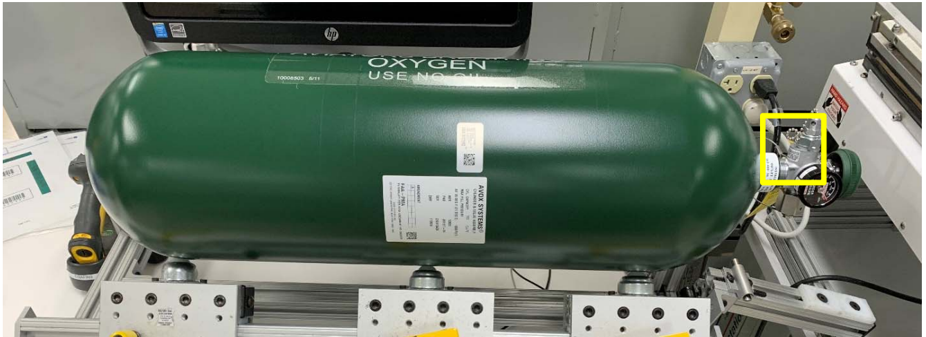
FIGURE 1 OVERVIEW OF CYLINDER AND VALVE ASSEMBLY
