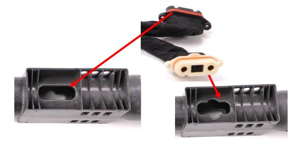
The ESC bracket of the T40 aircraft arm has different shapes of slots on both sides. Make sure that the side with the "petal" shape slot needs to face downwards, and the aircraft ESC composite cable connector should be passed through the slot.
