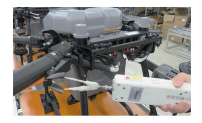
After the aircraft arm lock is replaced, fasten the lever. The tension value needs to be tested (acceptable tension range:  $90 \pm 10N$ ).
