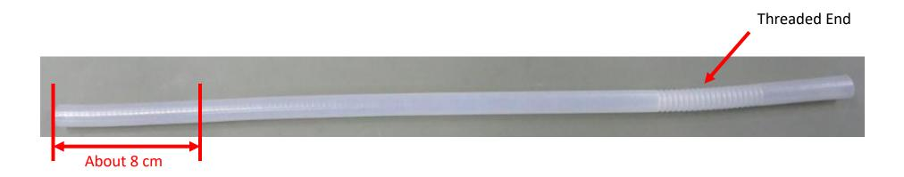
To use the T40 spray rod hose with the T20P drone, **the non-threaded end part** (close to the centrifugal motor) of the hose should be cut off about 8 cm. Otherwise, the spray rod hose cannot be connected to the aircraft arm hose.
