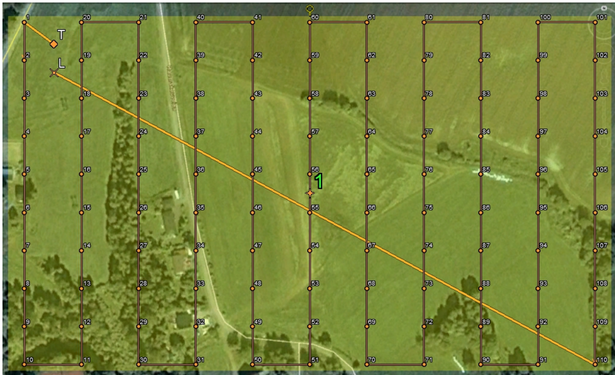
AreaWaypoint (AWP). Example covers 35 acres (~140,000 sq. meters) with 110 photopoints. Shown are the Takeoff (T) and Landing (L) waypoints which, when combined with the AWP, comprise an example of a complete Kestrel 3 Autopilot flight plan.
