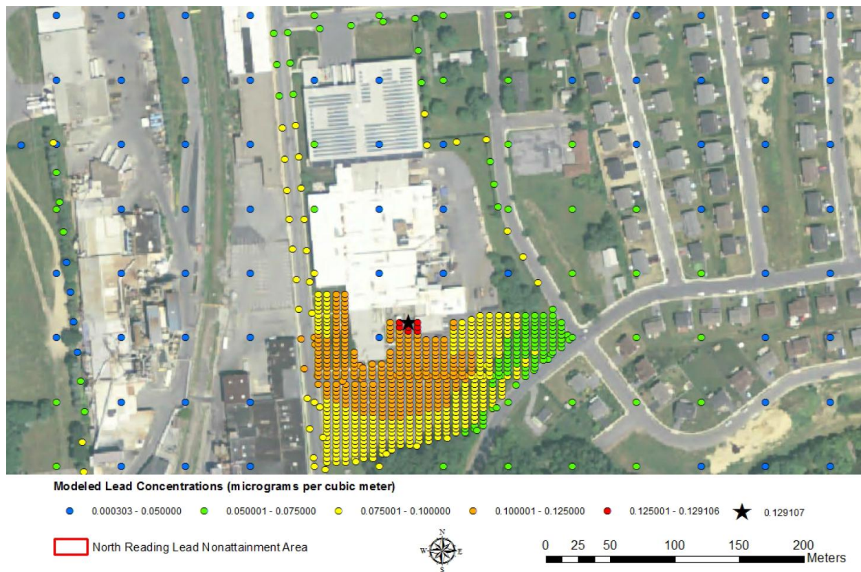
Figure 9: Future Case Modeling Predicted Lead Concentration in the North Reading Nonattainment Area Further Zoomed Into Area of Maximum Impact - Yuasa Parking Lot
