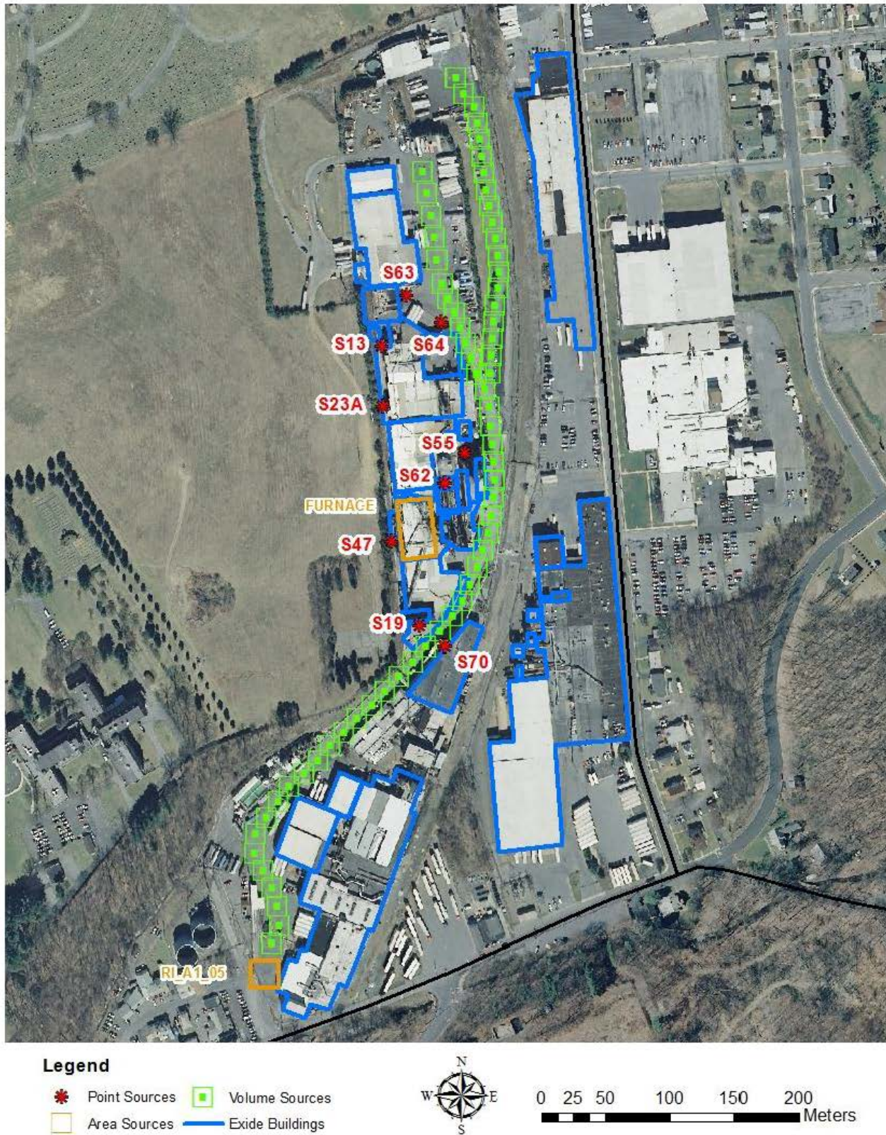
Figure 3: Exide's Lead Emission Sources and Building Configuration
