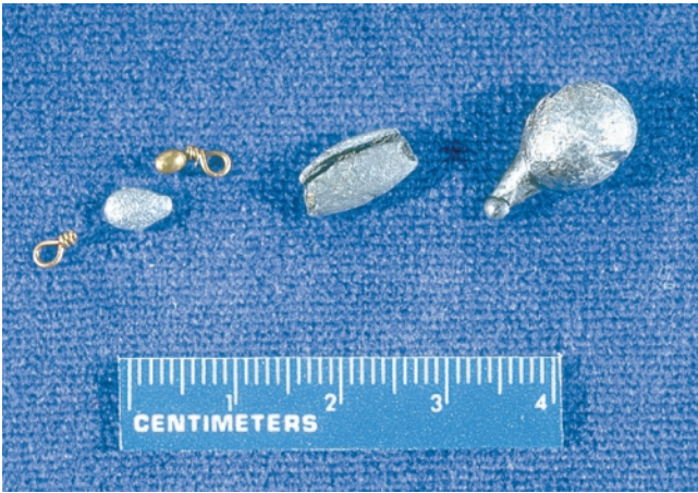
Figure 43.20 Fishing weights found in the stomachs and gizzards of birds that died from lead poisoning.
