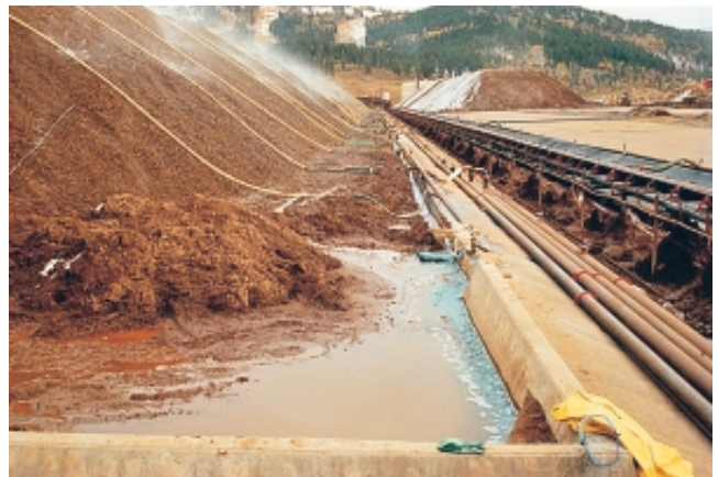
Figure 46.3 Heap leach pads at a mine that uses cyanide in the gold-extraction process. The water puddling at the base of the pad in the foreground contains cyanide.
