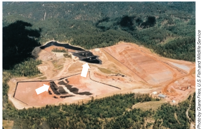
Figure 46.2 Aerial view of a heap leach mine. Note the open ponds of water (arrows).
