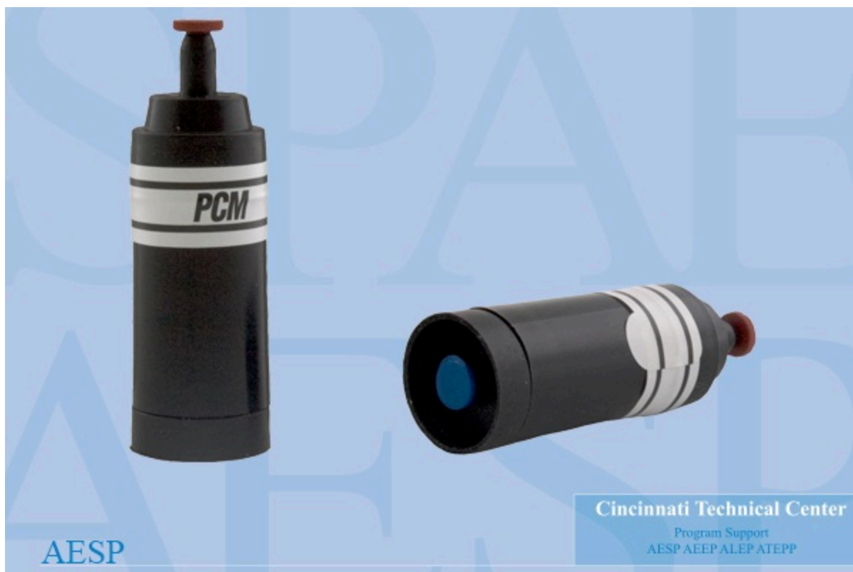
Figure 5. 0.8- \mu m pore size, 25-mm diameter MCEF cassette in an electrically conductive cassette assembly with 50-mm extension cowl. The end cap of the cassette visible on the right includes a blue Luer type plug. The entire end cap must be removed to allow open face sampling.
