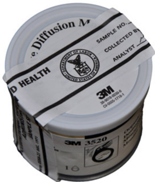
Figure E-7. Correctly sealed 3M passive monitor
