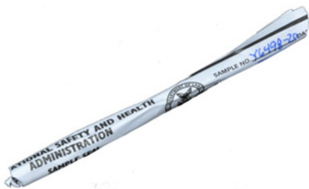
Figure E-1. Correctly sealed charcoal tube inside Form OSHA-21
