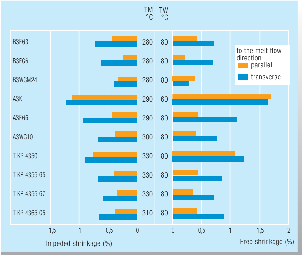
Fig. 46: Free and impeded shrinkage of Ultramid; sheet measuring 110 x 110 x 2 mm with film gate, holding pressure 500 bar, measured after storage for 1 h at 23 °C
