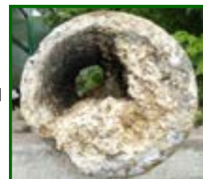
Sewer pipe clogged with grease
