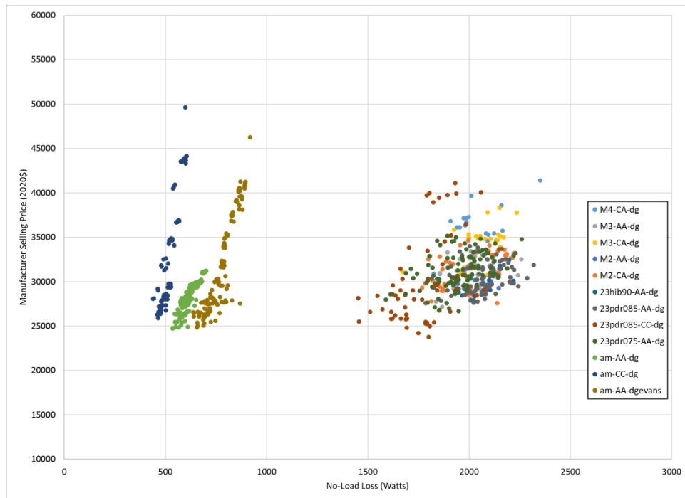
Figure 5A.2.13 Plot of Manufacturer Selling Price and No-Load Loss for RU5
