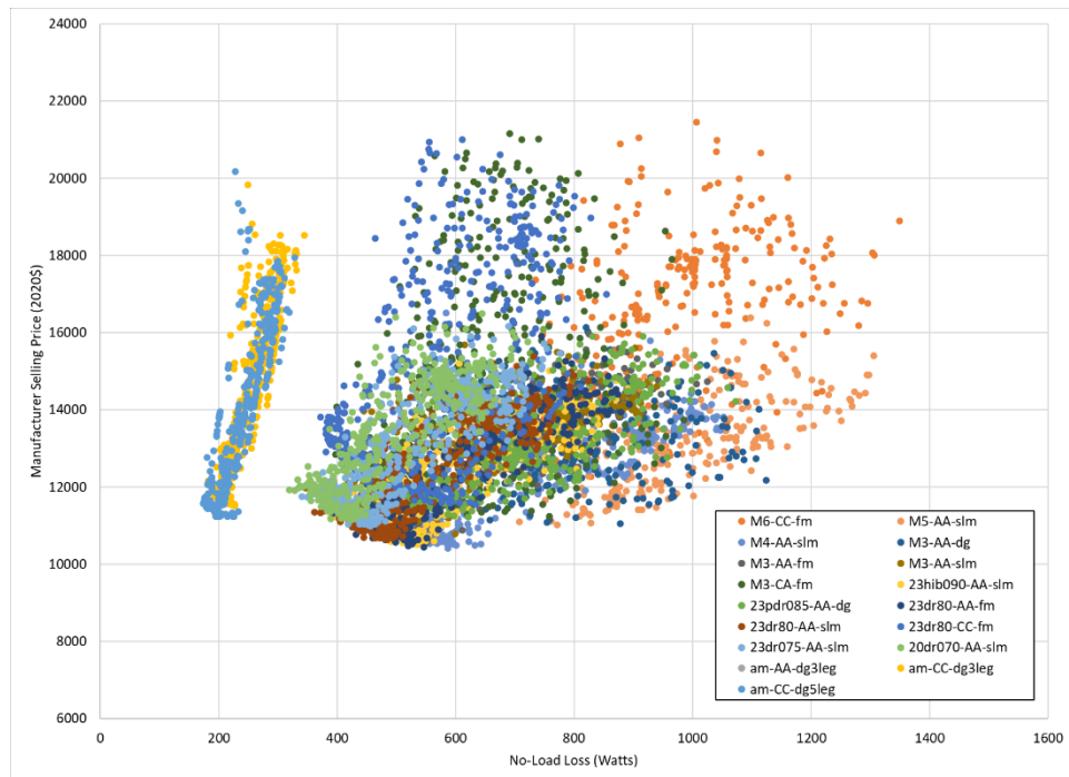
Figure 5A.2.25 Plot of Manufacturer Selling Price and No-Load Loss for RU9
