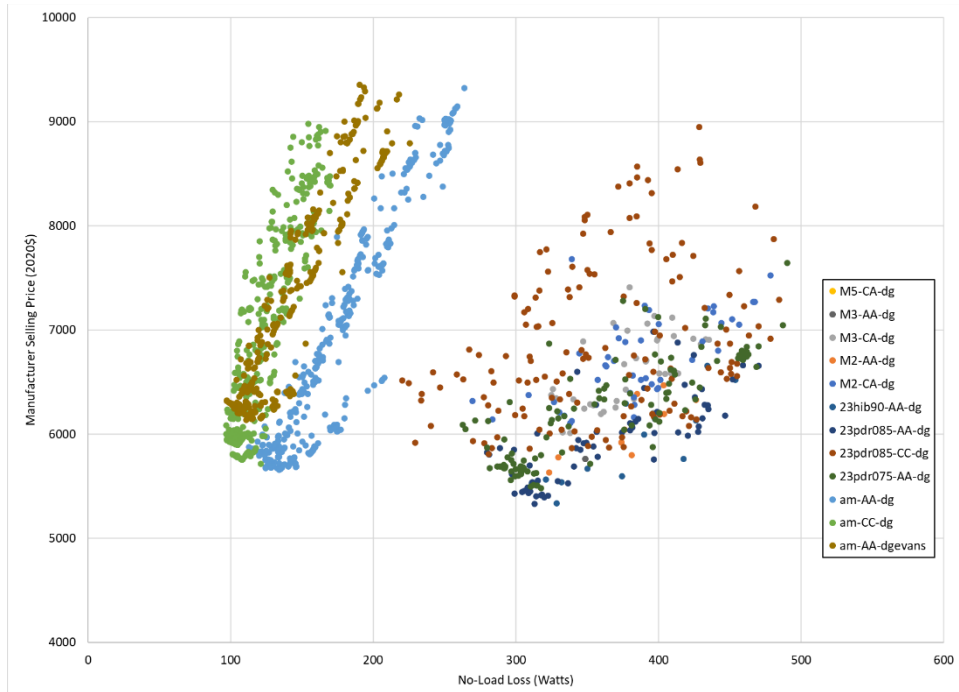
Figure 5A.2.10 Plot of Manufacturer Selling Price and No-Load Loss for RU4
