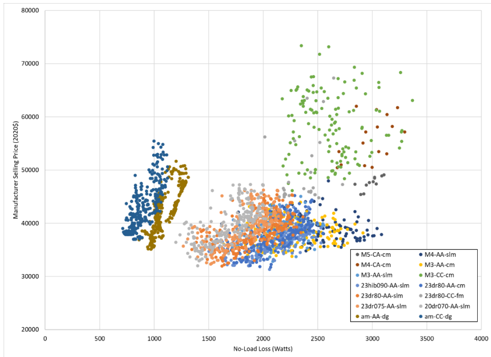
Figure 5A.2.28 Plot of Manufacturer Selling Price and No-Load Loss for RU10
