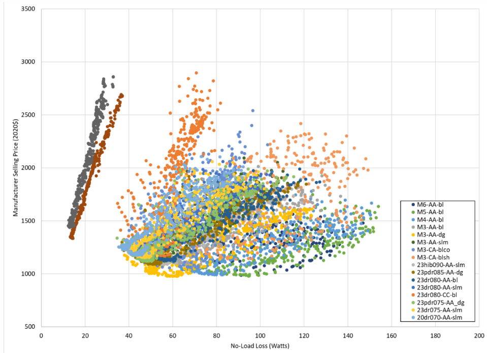
Figure 5A.2.16 Plot of Manufacturer Selling Price and No-Load Loss for RU6
