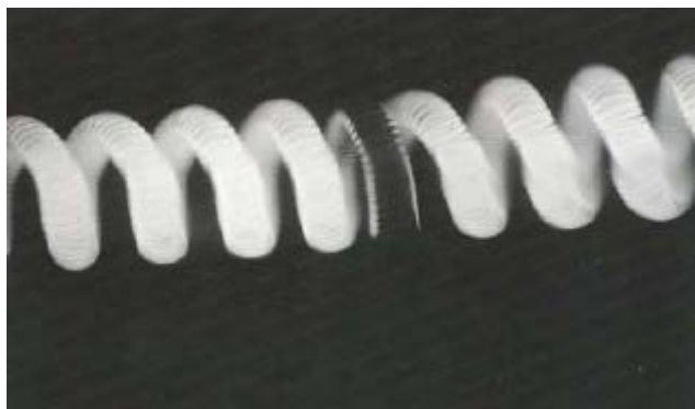
Figure 8D.1.1 Filament after Hot Shock; Shorted Coils Visible 3
