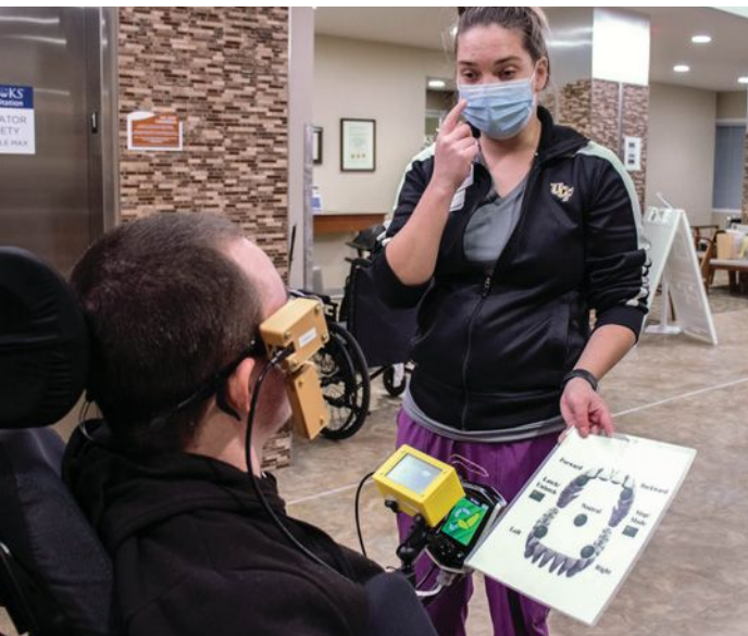
A study participant, left, learns how to use the MagTrack controller to drive a power wheelchair.
