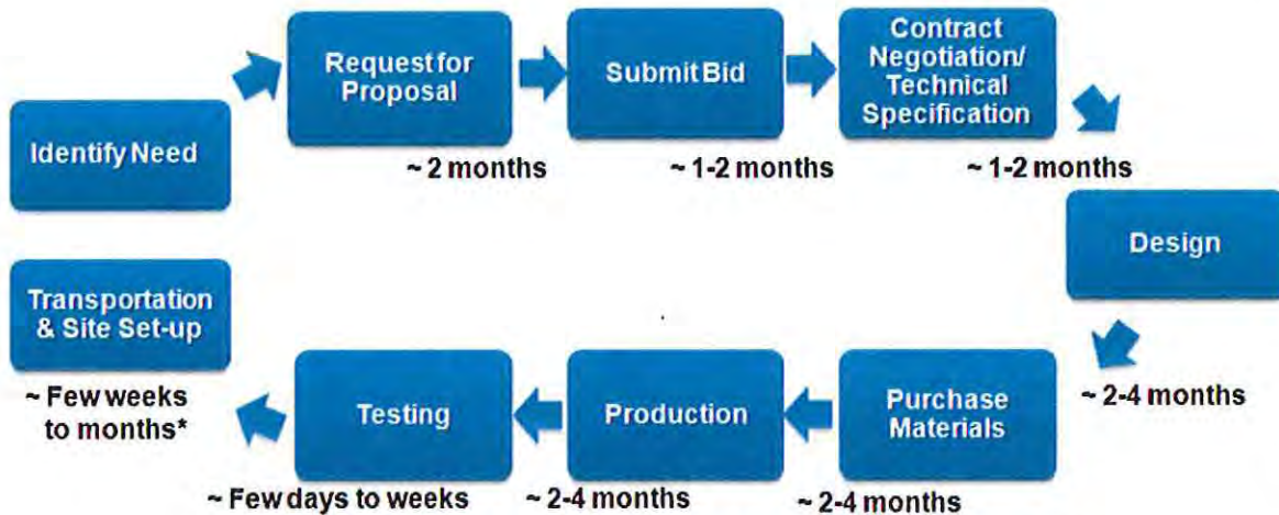
Figure 4: Representative Transformer Manufacturing Timeline
