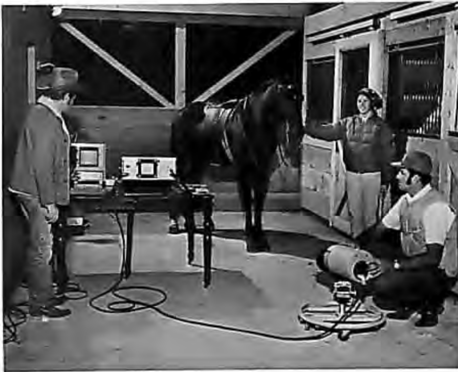
Figure 1. Placement of thermography equipment for examination of dorsal pastern. Camera placement is 6-10 feet from horse.
