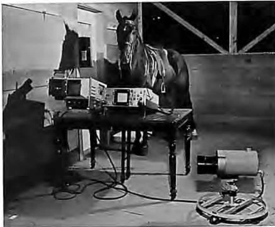
Figure 2. Thermography equipment including; camera, black and white monitor, color monitor.
